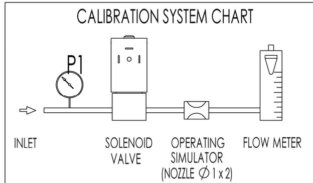
**V164B90 – ZE30C/ZE30A (orifice size=1.6mm)**
